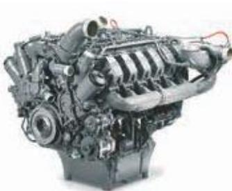
The 24.2 liter D2862 V12 engine from MAN is standard on the new JAGUAR 980 and 970 models and meets EPA Tier 4 emissions requirements.
