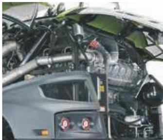
A new shielding design on the JAGUAR 980 and 970 increases airflow for the engine.
